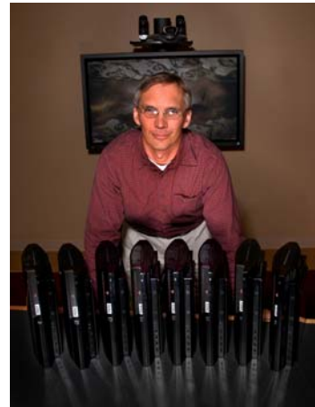
Using eight Sony Playstation 3 units, Dr. Frank Mueller built a supercomputing cluster capable of high-performance computing and running the latest in computer
